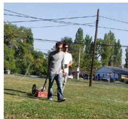
Figure 2: Ground Penetrating Radar (GPR) survey (Copyright: Dr Caroline Sturdy Colls)
